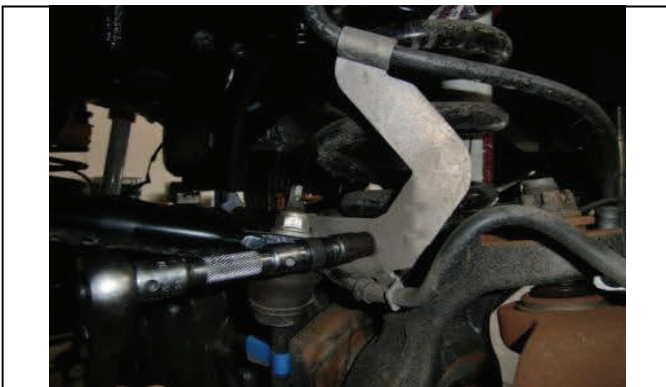
Disconnect brake line support bracket
