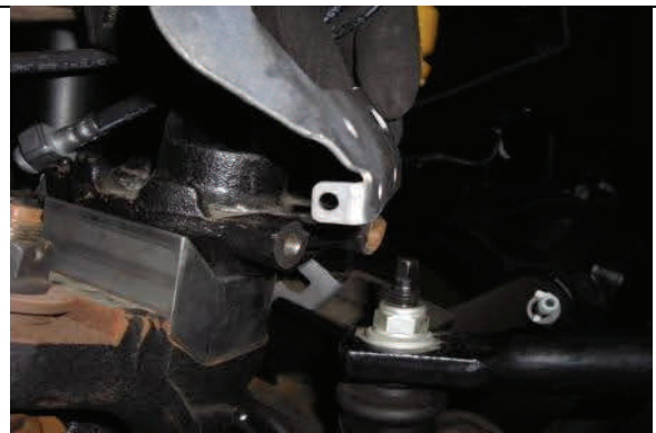
Then reconnect vacuum line and clip and reattach bracket
