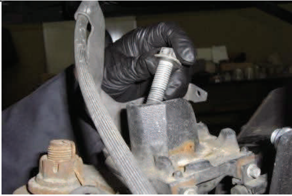
Remove bolt from middle of spring perch
