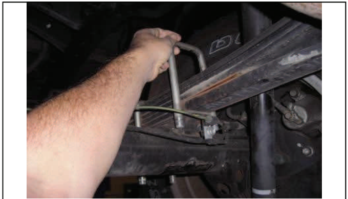
Carefully lower axle and remove u-bolts
