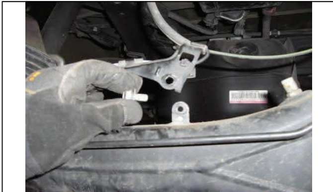
Disconnect ABS wiring brackets from axle.
