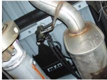
1. Apply a penetrating lubricant liberally to all exhaust fasteners, hangers and rubber isolators.
