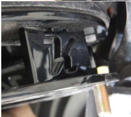
3. Now that the spacer is installed on the air bag, locate the grade 8 1/4-20-1" bolts. Use these to bolt the spacer to the axle. Torque to 30 ft/lbs
