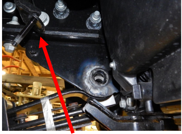
The radiator bolt in gusset removed on drivers side
