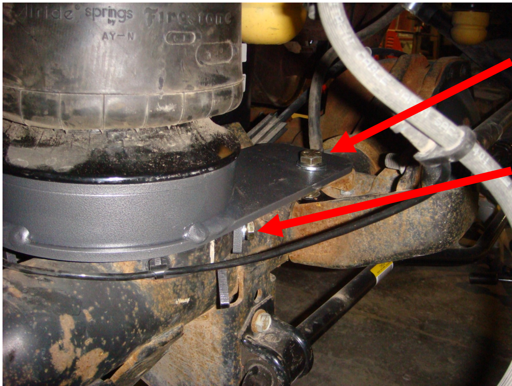
1/2 x 1 1/2" bolt uses tab nut on bottom
