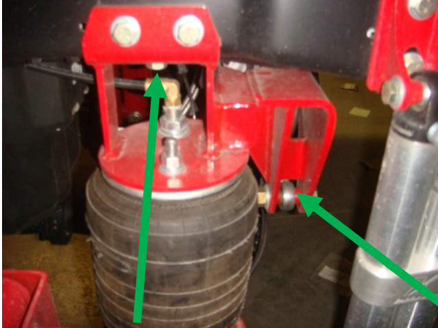
1/2x2" bolts Two in side of frame and one in the bottom PASSENGER SIDE PICTURED
