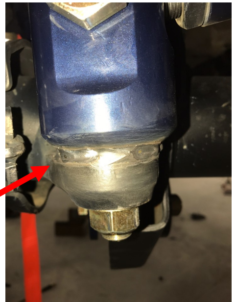
Lower pan hard bar mount and axle ground
