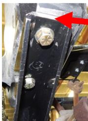
*Grind this area where you are going to weld the bracket to the frame*
