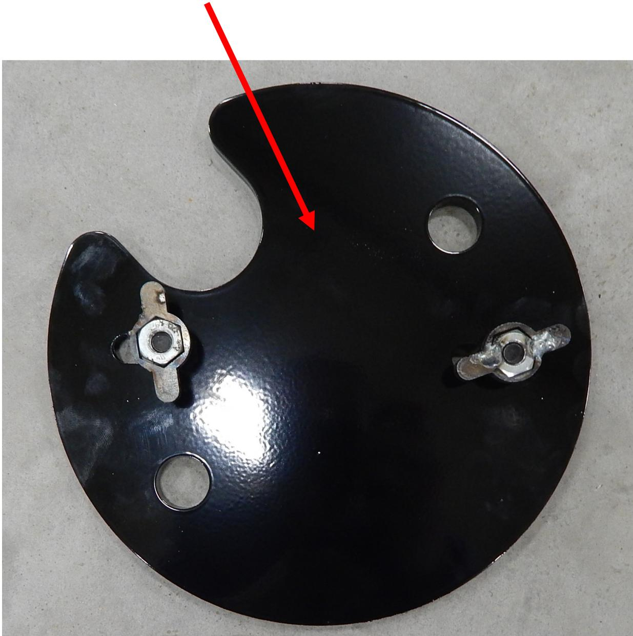
6. Locate the passenger side upper air bag mount (Part # 69049). It fastens to the bottom of the frame with the 3/8 x 1" counter sunk bolts, factory hitch with the 5/8 x 2" bolts and side of the frame with two 5/8 x 4" bolts. Torque the 3/8" bolts to 45 ft./lbs. and the 5/8" bolts to 155 ft./lbs.
