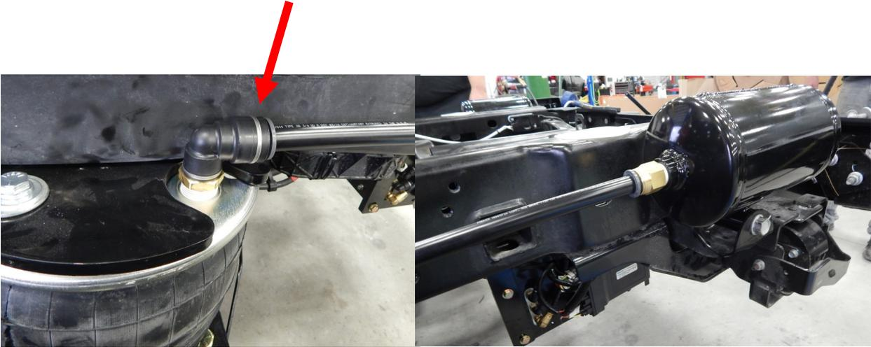
10. Locate the track bar/panhard bar (Part # 69470). It fastens to the upper and lower pan hard bar mounts with the 3/4 x 4" bolts. Use the spacers (Part # 18785 & # 18786) to center the heim ends up in the mounting brackets. Torque the 3/4" bolts to 200 ft./ lbs.
