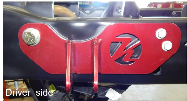
Use the two factory bolts on the drivers side and four bolts on the passenger side.
