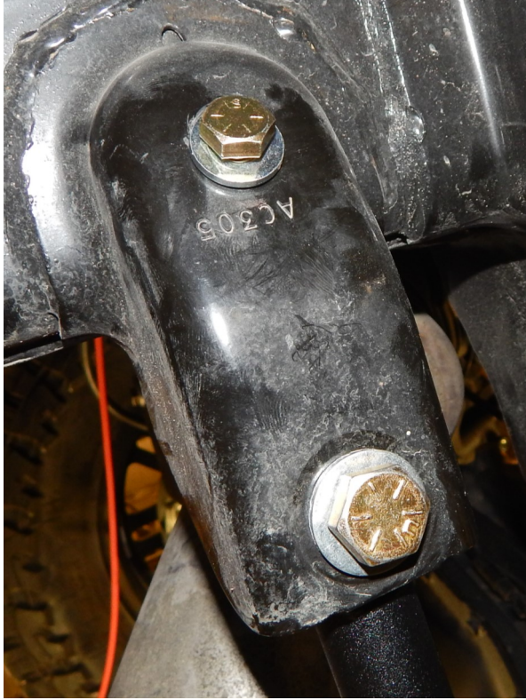
End link installed into the factory mount using 1/2 x 3" bolts and the 3/8 x 1 1/4" bolts
