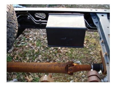
15. Locate the air tank. Mount find an area on the frame to mount it. Make sure the drain plug is facing straight down.
