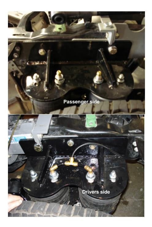
10. Locate the pan hard bar. The pan hard bar fastens into the lower air bag mount on the passengers side and into the upper pan hard bar mount fastened on the inside of the drivers side frame rail. Fasten in place using the 3/4x4" bolts.
