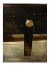
5. Locate the lower bag mounts The driver's side mount is the one with the pan hard bar ears. Lo-
