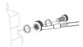
HINT: Install with new copper washers as indicated above. Brake line will only install with the "step" engaged on protruding portion of caliper. This prevents the brake line from rotating and ensures it will not contact the tire.
