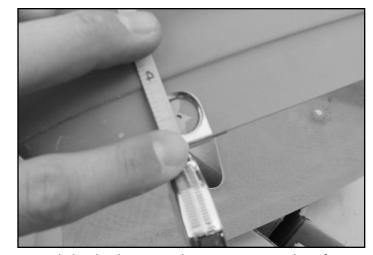
4) Mark the dead center with a permanent marker of where the clips fit onto the body panels. Measure twice, drill once!
