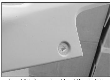
14) Now drill the front portion of the tail (if applicable) and mount tail section to bike. **Measure twice**, drill once!
