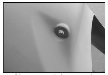
**13)** Drill the mounting bosses for the tail section in the center, **Measure twice, drill once!**
