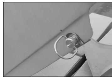
**10)** Check to make sure the "d-rings" fit through the body panel and clips, adjust if necessary.
