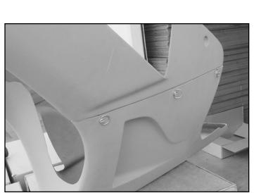
9) Check to make sure the "d-rings" fit through the body
