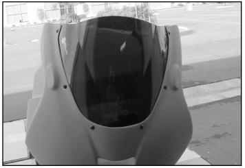
12) Mark and drill windscreen on bodywork, mount screen to upper fairing. DO NOT drill the upper fairing stay yet! **Measure twice, drill once!**
