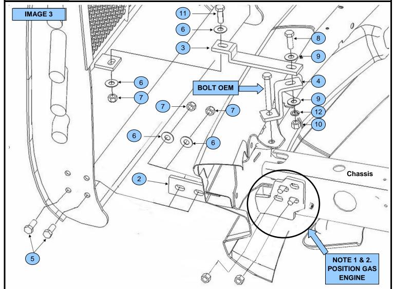
**Note 1**. Use the existent bolts to fix the bracket, if the vehicle doesn't have tow hooks, use the  $1/2 \times 1 \cdot 1/2$ " bolts in the hardware kit.
