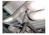
4. INSTALL DRIVERS SIDE OVER AXLE TAILPIPE # C INTO MUFLER 1 ½" TO 2" USE CLAMP # H TO SECURE PIPE TO MUFFLER. DO NOT TIGHTEN.
