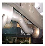
1. TO REMOVE STOCK EXHAUST UN-BOLT IT FROM THE CLAMP LOCATED JUST BEHIND THE CATALITIC CONVERTER. CUT OFF YOUR STOCK TAILPIPE AND REMOVE. LEAVE ALL RUBBER GROMMETS IN PLACE. USE WD-40 TO AID IN REMOVAL OF EXHAUST AND HANGERS.
