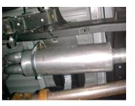
3. INSTALL BAND CLAMP # G INTO RUBBER GROMMETS LOCATED ABOVE THE REAR AXLE AND ATTACH WITH BOLT KIT #M. DO NOT TIGHTEN. INSTALL MUFFLER # B THROUGH BAND CLAMP AND ONTO HEADPIPE. USE CLAMP # L TO SECURE MUFFLER TO HEADPIPE. DO NOT TIGHTEN.
