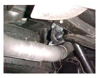
5. INSTALL PASSENGER SIDE OVERAXLE TAILPIPE # D INTO MUFFLER 1 ½" TO 2" INSERT WELDED HANGER INTO RUBBER GROMMET. USE CLAMP # H TO SECURE PIPE TO MUFFLER. DO NOT TIGHTEN.
