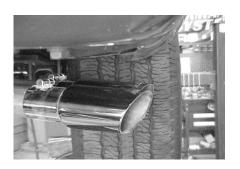
INSTALL TAILPIPES#C, D USING CLAMP#G TO ATTACH TO MUFFLER. BOLT KIT#H TO CONNECT BOTH THE TAILPIPES TOGETHER. THE TAB ON THE DRIVERSIDE TAILPIPE WILL BE ON TOP. TIGHTEN ALL CLAMPS AND HANGERS. NOW INSTALL YOUR STAI NLESS STEEL TIPS TO YOUR DESIRED LOOK. USE ANY ALUMINUM OR STAINLESS STEEL CLEANER TO POLISH YOUR TIP.
