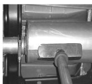
NEXT, CONNECT HEADPIPE# A TO THE STOCK FLANGE USING GASKET #I. RE-USE STOCK NUTS AND GASKET. CONNECT THE MUFFLER # B TO HEADPIPE USING CLAMP# F. SUPPORT THE MUFFLER WITH A JACKSTAND. THE INLET WILL BE AT APPROXIMATELY 6 O'CLOCK. INSERT WELDED HANGER INTO RUBBER GROMMET.
