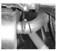
LAYOUT THE GIBSON EXHAUST AS SHOWN ON YOUR MANUAL. COMPARE THE PIPE NUMBERS TO THE MANUAL NUMBERS. MAKE SURE THEY ALL MATCH. THEN, CUT THE STOCK TAILPIPE OFF JUST AFTER THE MUFFLER FOR EASY REMOVAL. AFTER CUTTING THE TAILPIPE, UNBOLT THE STOCK HEADPIPE AND REMOVE THE WHOLE SYSTEM. LEAVE ALL RUBBER GROMMETS IN PLACE. YOU WILL REUSE STOCK FLANGE BOLTS AND GASKETS.
