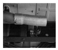
2. SLIP HEADPIPE #A ONTO THE FACTORY HEADPIPE. USE CLAMP #H TO ATTACH IT. DO NOT TIGHTEN.
