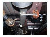
TO REMOVE YOUR STOCK REMOVE IT FROM THE CL/ LOCATED JUST IN FRONT MUFFLER REMOVE HANGE RUBBER GROMMETS BY PU EXHAUST TOWARDS THE THE VEHICLE, USE WD-40 REMOVAL, LEAVE GROMME PLACE.
