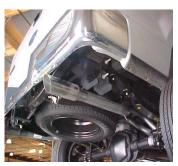
INSTALL PASSENGER SIDE TAILPIPE # C INTO MUFFLER 1 ½" TO 2". INSERT WELDED HANGER INTO RUBBER GROMMET, USE CLAMP # H TO SECURE PIPE TO MUFFLER. DO NOT TIGHTEN. ROTATE PIPE TOWARDS DRIVERSIDE.
