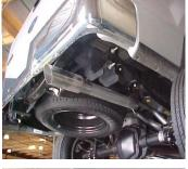
INSTALL YOUR STAINLESS TIPS TO YOUR DESIRED LOOK, THEN GO BACK AND TIGHTEN ALL CLAMPS. ROTATE SYSTEM FOR BEST CLEARANCE BEFORE TIGHTENING.
