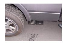
INSTALL STAINLESS TIPS, CLAMP DOWN. TO CLEAN YOUR STAINLESS TIPS USE ANY STAINLESS CLEANER OR A SCOTCH BRITE PAD. NOW GO AND TIGHTEN ALL CLAMPS, NUTS AND BOLTS. START FROM THE FRONT AND WORK BACK.
