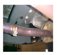
TO REMOVE YOUR STOCK EXHAUST, REMOVE IT FROM THE CLAMP LOCATED JUST IN FRONT OF THE MUFFLER REMOVE HANGERS FROM RUBBER GROMMETS BY PULLING EXHAUST TOWARDS THE REAR OF THE VEHICLE, USE WD-40 TO AID IN REMOVAL, LEAVE GROMMETS IN PLACE. LEAVE YOUR FACTORY CLAMP ON PIPE YOU WILL RE-USE IT.
