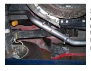
**5.** Install the passenger side overaxle tailpipe #C into the muffler 1½"-2". Use clamp #H to secure tailpipe to muffler. DO NOT TIGHTEN. Insert hanger into rubber grommet.
