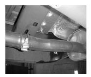
TO REMOVE YOUR STOCK EXHAUST, REMOVE IT FROM THE CLAMP LOCATED JUST IN FRONT OF THE MUFFLER REMOVE HANGERS FROM RUBBER GROMMETS BY PULLING EXHAUST TOWARDS THE REAR OF THE VEHICLE, USE WD-40 TO AID IN REMOVAL, LEAVE GROMMETS IN PLACE.
