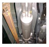
INSTALL MUFFLER # B ONTO HEADPIPE 1  $\frac{1}{2}$ " TO 2". USE A JACK STAND TO HOLD UP THE MUFFLER. OUTLETS SHOULD BE ON THE TOP.
