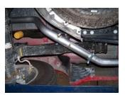
**4.** Install the passenger side overaxle tailpipe #C into the muffler  $1\frac{1}{2}$ "-2". Use clamp #H to secure tailpipe to muffler. DO NOT TIGHTEN. Insert hanger into rubber grommets.
