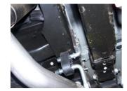
**5.** Install hanger #I into hole located approximately 19" from the rear of the frame. Use bolt kit #J to secure. DO NOT TIGHTEN. Install rubber grommet
