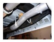
**2.** Install head pipe #A onto your existing stock front pipe and attach with clamp #G. Use a jack stand to support the converter. Insert welded hanger into rubber grommet.
