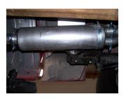
3. Install muffler #B onto head pipe #A 11/2"-2" with the louvers facing towards the converter. Use a jack stand to support the muffler. Use clamp #G to secure the muffler to the headpipe. Do not tighten. Muffler inlet is looking into the louvers.
