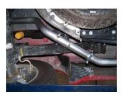
4. Install the passenger side overaxle tailpipe #C into the muffler 11/2"-2". Use clamp #H to secure tailpipe to muffler. DO NOT TIGHTEN. Insert hanger into rubber grommets.
