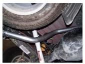
6. Install the driverside overaxle tailpipe #D into the muffler 11/2-2". Use clamp #H to secure. DO NOT TIGHTEN. Rotate until it meets with the rubber grommet, use clamp #H to hold pipe. DO NOT TIGHTEN.
