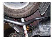
**6.** Install the driverside overaxle tailpipe #D into the muffler 1½-2". Use clamp #H to secure. DO NOT TIGHTEN. Rotate until it meets with the rubber grommet, use clamp #H to hold pipe. DO NOT TIGHTEN.
