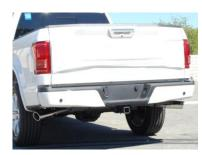
INSTALL YOUR STAINLESS TIPS AND CUT YOUR EXIT PIPES TO YOUR DESIRED LOOK AND LENGTH\*\* THEN GO BACK AND TIGHTEN ALL CLAMPS, ROTATE SYSTEM FOR BEST CLEARANCE BEFORE TIGHTENING.
