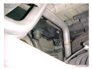
INSTALL PASSENGER SIDE TAILPIPE # C INTO MUFFLER 1<sup>1</sup>/<sub>2</sub>" TO 2". INSERT WELDED HANGER INTO RUBBER GROMMET, USE CLAMP # H TO SECURE PIPE TO MUFFLER, DO NOT TIGHTEN. ROTATE PIPE TOWARDS DRIVERSIDE.
