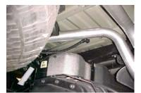
INSTALL DRIVERS SIDE TAILPIPE # D INTO MUFFLER 1 불" TO 2". INSERT WELDED HANGERS INTO RUBBER GROMMETS. USE CLAMP # H TO SECURE PIPE TO MUFFLER, DO NOT TIGHTEN.
