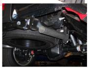
INSTALL PASSENGER SIDE TAILPIPE # C INTO MUFFLER  $1\frac{1}{2}$ " TO 2". INSERT WELDED HANGER INTO RUBBER GROMMET, USE CLAMP # H TO SECURE PIPE TO MUFFLER. DO NOT TIGHTEN. ROTATE PIPE TOWARDS DRIVERSIDE.
