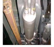
INSTALL MUFFLER # B ONTO HEADPIPE 1  $\frac{1}{2}$ " TO 2". USE CLAMP '# G TO SECURE MUFFLER TO HEADPIPE. DO NOT TIGHTEN. USE A JACK STAND TO HOLD UP THE MUFFLER. OUTLETS SHOULD BE LEVEL.
