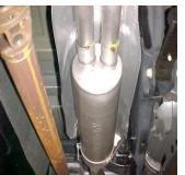
INSTALL MUFFLER # B ONTO HEADPIPE 1 ½" TO 2". USE CLAMP '# G TO SECURE MUFFLER TO HEADPIPE. DO NOT TIGHTEN. USE A JACK STAND TO HOLD UP THE MUFFLER. OUTLETS SHOULD BE LEVEL.
