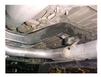
INSTALL Y-PIPE # A & P ONTO STOCK FLANGES USE YOUR STOCK HARDWARE TO SECURE INSERT WELDED HANGER INTO RUBBER GROMMET, DO NOT TIGHTEN.
