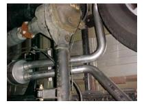
NEXT, INSTALL DRIVERS SIDE TAILPIPE # D INTO MUFFLER 1 ½" -2". USE CLAMP # J TO SECURE PIPE INTO MUFFLER, DO NOT TIGHTEN. ROTATE PIPE UNTIL IT MAKES CONTACT WITH HANGER # K USE CLAMP # J TO HOLD PIPE UP. NEXT, INSTALL EXIT PIPES # F ONTO TAILPIPE, DO NOT TIGHTEN, REPEAT THIS STEP FOR THE PASS. SIDE, USING TAILPIPE # E.
