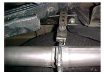
ON THE DRIVERS SIDE MEASURE APPROX. 17" FROM THE REAR OF THE FRAME USE THIS 1" HOLE TO BOLT HANGER # K USING THE TOP HOLE ON HANGER & HARDWARE PROVIDED, REPEAT FOR PASSENGER SIDE.
