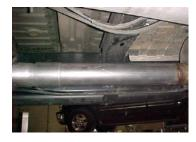
INSTALL MUFFLER # C ONTO YOUR RESONATOR 1 ½" -2". USE CLAMP # I TO SECURE MUFFLER TO THE PIPE, DO NOT TIGHTEN.
