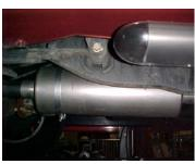
INSTALL EXTENSION PIPE #O ONTO HEADPIPE.
