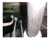
INSTALL BAND CLAMP # H ONTO MUFFLER, INSERT HANGER INTO RUBBER GROMMET, USE BOLT KIT PROVIDED, DO NOT TIGHTEN.
