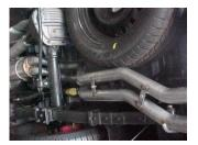
Install the driver side over axle tailpipe #D into the muffler 1-1/2" to 2". Use clamp #H to secure tailpipe to muffler. Use bolt kit #I to secure tailpipes #D & E together. Driver side tailpipe will have tab on bottom. Do not tighten.
