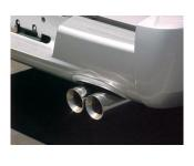
Install the stainless tips. Clamp down. To clean your stainless tips use any stainless cleaner or a Scotch Brite pad. Now go back and tighten all clamps, nuts and bolts. Start from the front and work back.
