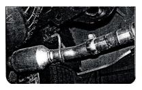
1. Disconnect the negative battery cable before removal of OEM exhaust. This will allow the computer to reset and recognize the new exhaust. Lay out the exhaust on the floor so it looks like the drawing and compare parts with manual.
