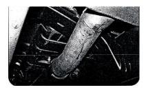
2. To remove the stock exhaust, remove it from the two bolt flange in front of the muffler. Do not discard you will re-use bolts. Disengage the welded hangers using WD-40 from the OEM rubber grommets. Do not damage or remove the rubber grommets as you will reuse them to mount your new system. Now, cut off tailpipe before and after rear axle for removal.
