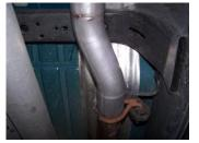
3. Install headpipe #A onto your existing stock headpipe and attach with clamp #I. Do not tighten. Use a jack stand to support the converter.
