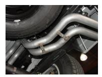
INSTALL PASSENGER SIDE TAILPIPE #D INTO MUFFLER AND ATTACH USING CLAMP #F. INSERT WELDED HANGER INTO RUBBER GROMMET. DO NOT TIGHTEN. USE BOLT KIT #I TO ATTACH THE TAILPIPES TOGETHER. DO NOT TIGHTEN. DRIVER SIDE TAILPIPE TABS WILL BE ON THE BOTTOM.
