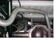
**INSTALL DRIVER SIDE** TAILPIPE #D INTO MUFFLER 1-1/2" TO 2" AND USE CLAMP #G TO SECURE THE MUFFLER. DO NOT TIGHTEN. USE CLAMP #G TO HOLD PIPE UP TO THE HANGER #F. DO NOT TIGHTEN.
