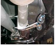
**INSTALL MUFFLER #B** ONTO HEADPIPE 1-1/2" TO 2". USE CLAMP #H TO SECURE THE MUFFLER TO THE HEADPIPE. DO NOT TIGHTEN. SLIDE BAND CLAMP #I ONTO THE MUFFLER AND INSERT THE WELDED HANGER INTO THE RUBBER GROMMET AND ATTACH WITH BOLT KIT #J.
