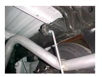
INSTALL HEADPIPE #A, YOU WILL NEED TO LINE UP THE TWO NOTCHES. USE FRONT HANGER #L TO SECURE PIPES TOGETHER AND INSERT HANGER INTO RUBBER GROMMET. DO NOT TIGHTEN.
