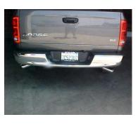
INSTALL THE STAINLESS TIPS. TO CLEAN TIPS USE ANY STAINLESS CLEANER AND A SCOTCH BRITE PAD. NOW GO BACK AND TIGHTEN ALL CLAMPS, NUTS AND BOLTS STARTING FROM THE FRONT AND WORKING BACK.
