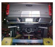
INSTALL EXIT PIPES #E, USE CLAMPS #G TO SECURE TO THE TAILPIPES.
