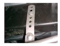
MEASURE 19 ½" FROM THE REAR OF THE FRAME AND USE THIS HOLE AND BOLT ON HANGER #H. USE THE 2<sup>ND</sup> HOLE FROM THE TOP.
