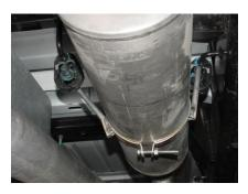
INSTALL MUFFLER #B ONTO HEADPIPE 1-1/2" TO 2". USE CLAMP #I TO SECURE THE MUFFLER TO THE HEADPIPE, DO NOT TIGHTEN. SLIDE BAND CLAMP #J ONTO THE MUFFLER AND INSERT THE WELDED HANGER INTO THE RUBBER GROMMET. ATTACH WITH BOLT KIT #L.
