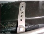
MEASURE 19 1/2" FROM THE REAR OF THE FRAME AND USE THIS HOLE AND **BOLT ON HANGER #G.** USE THE 2<sup>ND</sup> HOLE FROM THE TOP.
