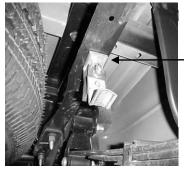
INSTALL HANGERS #G TO BOTTOM OF FRAME RAIL IN TEXISTING HOLE APPROXIMATELY 19 1/4" FROM REAR OF FRAME. USE NUT AND BOLT SUPPLIED.
