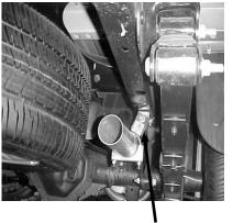
UNBOLT AND REMOVE STOCK REAR HANGER ON THE PASSENGER SIDE FRAME RAIL. INSTALL HANGERS # HTO THE BOTTOM OF FRAME RAIL IN EXISTING HOLE APPROX. 22 .5" FROM THE REAR OF THE FRAME, USE NUT AND BOLT THAT ARE SUPPLIED. REPEAT THIS SAME PROCEDURE ON DRIVERS SIDE. HANGER # H WILL AIM TOWARDS THE REAR OF THE VEHICLE.
