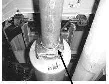
INSTALL HANGER # 6 IN FRONT OF THE MUFFLER AND INSERT INTO THE STOCK RUBBER GROMMETS. THEN INSTALL MUFFLER #B WITH INLET TOWARDS THE FRONT OF THE VEHICLE. USE A JACK STAND TO SUPPORT MUFFLER. DO NOT TIGHTEN.
