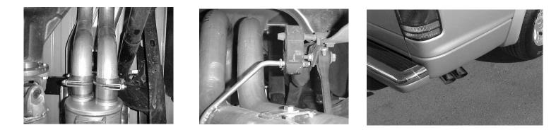
INSTALL PASSENGER OVERAXLE TAILPIPE #B INTO THE REAR OF THE MUFFLER USING CLAMP # E TO ATTACH TAILPIPE TO MUFFLER. INSTALL DRIVERSIDE OVERAXLE TAILPIPE #C. INSERT WELDED HANGER INTO RUBBER GROMMET. ATTACH HANGER TO MUFFLER. ATTACH TAILPIPES TOGETHER USING BOLT KIT # H. DRIVERSIDE TAILPIPE #C BRACKET SHOULD BE ON TOP OF PASSENGER TAILPIPE #B BRACKET. DO NOT TIGHTEN.
