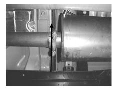
DO NOT REMOVE EXTENSION PIPE BETWEEN MUFFLER AND CATALYTIC CONVERTER. REMOVE THE FIRST CLAMP IN FRONT OF YOUR MUFFLER, THEN REMOVE STOCK EXHAUST. USE WD-40 ON HANGERS FOR EASIER REMOVAL.
