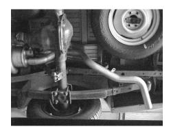
INSTALL PASSENGERSIDE OVERAXLE TAILPIPE #B INTO MUFFLER AT LEAST 1 ½"TO 2". USE CLAMP #E TO SECURE IT. DO NOT TIGHTEN. INSERT WELDED HANGER INTO RUBBER GROMMET.
