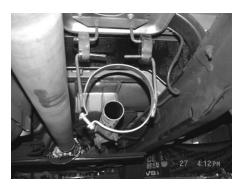
INSTALL THE BAND CLAMP #G INTO FACTORY GROMMETS BEHIND THE STOCK HEADPIPE. ATTACH WITH BOLT KIT #I. NEXT, SLIDE MUFFLER THROUGH THE BAND CLAMP WITH THE INLET TOWARDS THE MOTOR. USE CLAMP #E TO SECURE MUFFLER TO THE STOCK PIPE. USE A JACK STAND TO SUPPORT THE MUFFLER. INLET HAS LOUVERS INSIDE FACING TOWARDS THE MOTOR. DO NOT TIGHTEN
