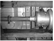
DO NOT REMOVE THE STOCK HEADPIPE. CUT 8" IN FRONT OF YOUR STOCK MUFFLER
