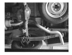
INSTALL PASSENGERSIDE OVERAXLE TAILPIPE #B INTO MUFFLER AT LEAST 1 ½"TO 2". USE CLAMP #E TO SECURE IT. DO NOT TIGHTEN. INSERT WELDED HANGER INTO RUBBER GROMMET.
