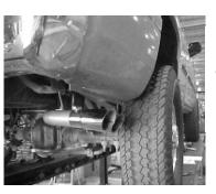
INSTALL THE STAINLESS TIPS. NOW GO BACK AND START AT THE FRONT AND TIGHTEN ALL CLAMPS AND HANGERS.
