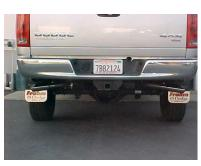
INSTALL THE STAINLESS TIPS. TO CLEAN TIPS USE ANY STAINLESS CLEANER AND A SCOTCH BRITE PAD. NOW GO BACK AND TIGHTEN ALL CLAMPS, NUTS AND BOLTS STARTING FROM THE FRONT AND WORKING BACK.
