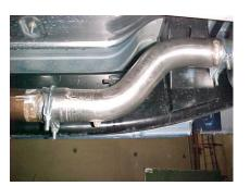
INSTALL HEADPIPE #A, YOU WILL NEED TO LINE UP THE TWO NOTCHES. INSERT WELDED HANGER INTO RUBBER GROMMET. USE CLAMP #G TO SECURE HEADPIPE TO THE STOCK PIPE. DO NOT TIGHTEN.
