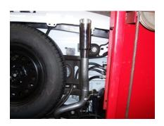
7.Install exit pipes #E onto tailpipes use clamp # F to secure together
